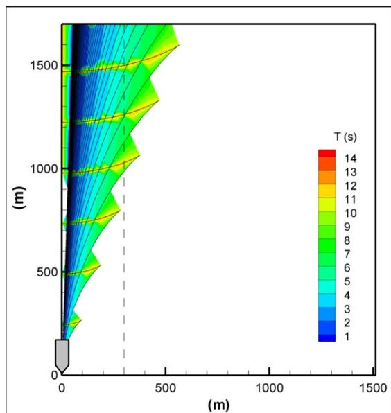
Figure 1a. Wake period for 38 knot vessel in infinite depth water
