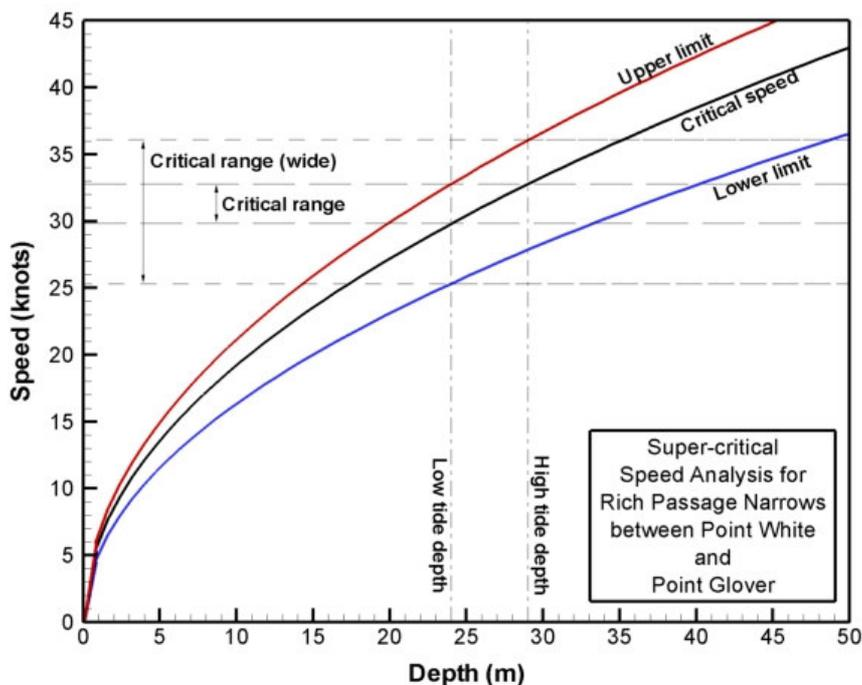
Figure 5. Critical speeds analysis for Rich Passage Narrows.
