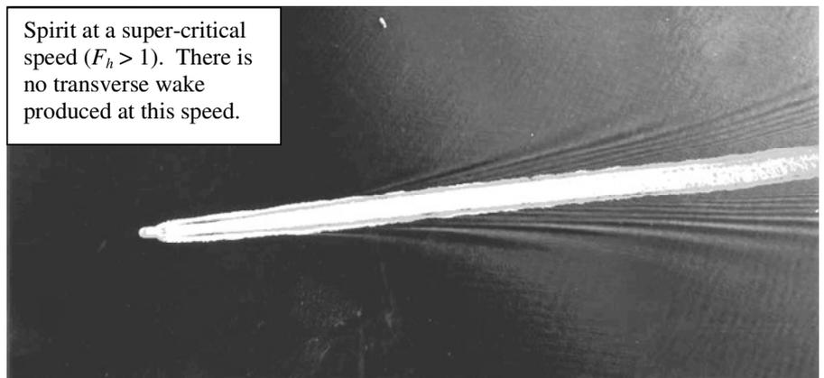
Figure. 4. Photograph of Spirit at a super-critical speed. Note only diverging wakes are present.
