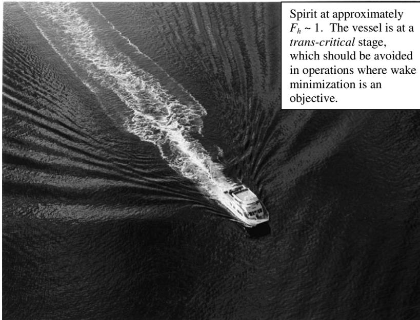
Spirit at approximately  $F_h \sim 1$ . The vessel is at a *trans-critical* stage, which should be avoided in operations where wake minimization is an objective.
