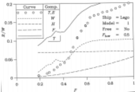
Figure 2 (a) Components of Resistance in Pure Theory - Model 1
