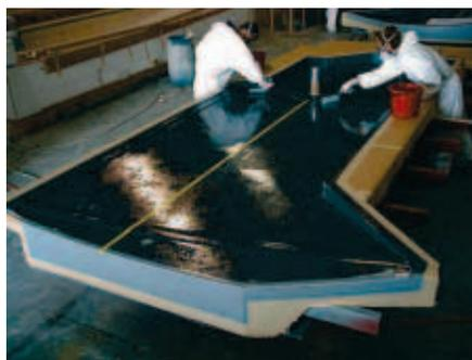
Figure 8: Strut Shell Mould
