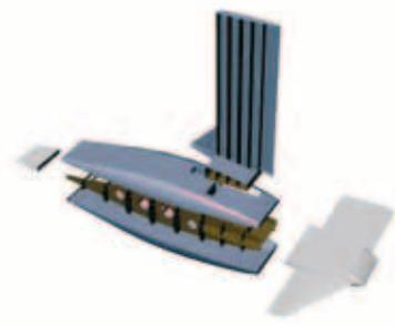
Figure 5: Exploded Basic Assembly
