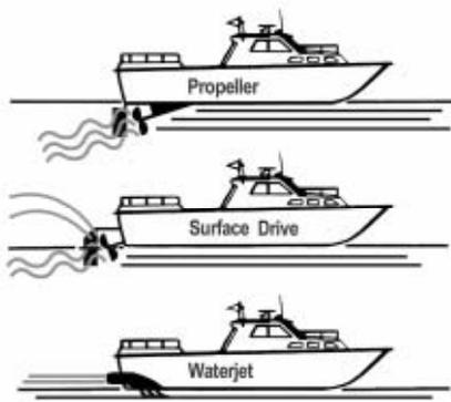
Fig. 1– Three Propulsion Systems
