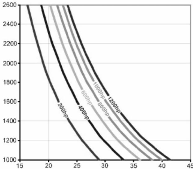
Fig. 3—Propeller Diameter/ HP/RPM
