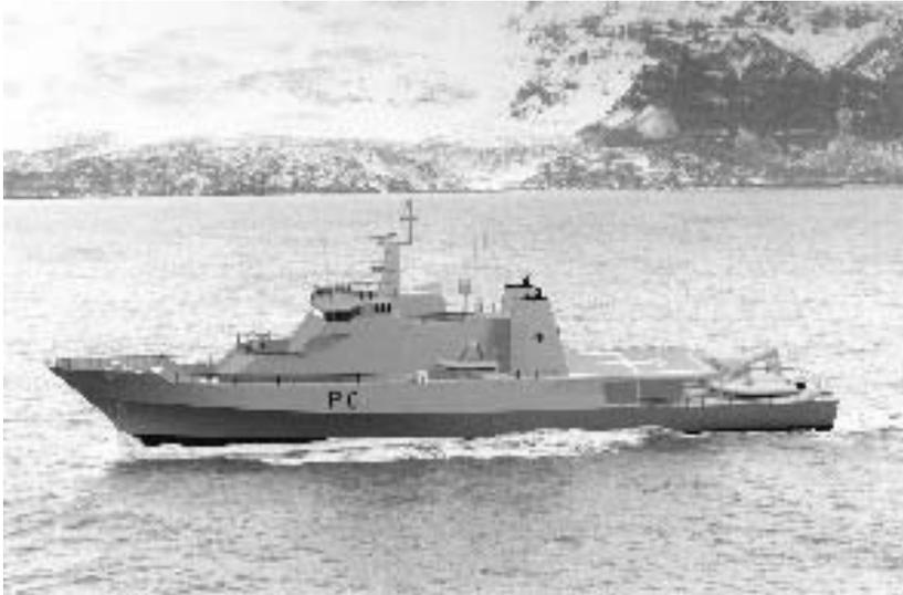
Tenix's proposed 1600 tonne displacement Offshore Patrol Vessel would be 85m long x 14m beam and capable of 22 knots with a range of up to 6,000nm. Accommodation on board for a core complement of 35, a flight of 10, and four government agency officers would be provided. Provision is also made for an additional 30 embarked personnel
