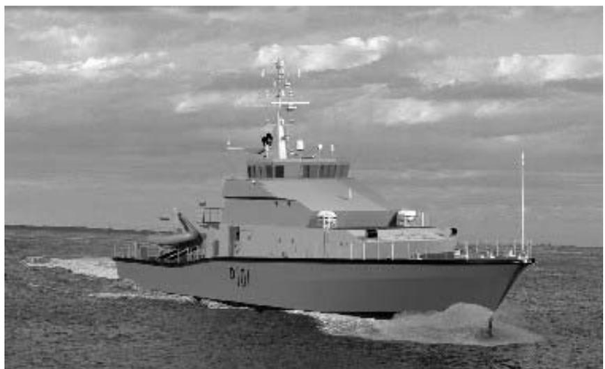
The proposed Inshore Patrol Vessel is 340 tonnes displacement, 55m long x 9m beam and capable of up to 25 knots, with a maximum range of 3000 nm. The ships will have accommodation for a core complement of 20 personnel plus provision for four government agency officers and 12 additional personnel.
