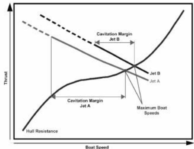
Fig 2.—Hull Resistance vs. Waterjet Thrust
