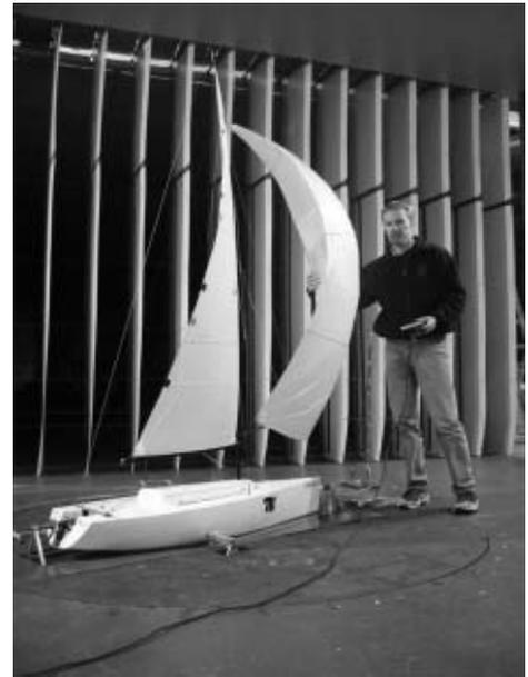
The typical mast height of a model in the TFWT is about 2.3 metres
