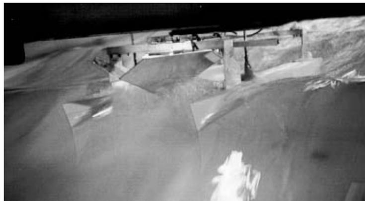
A typical semi captive model test. In this instance the model is being tested with a Vee shaped cross deck bow structure
