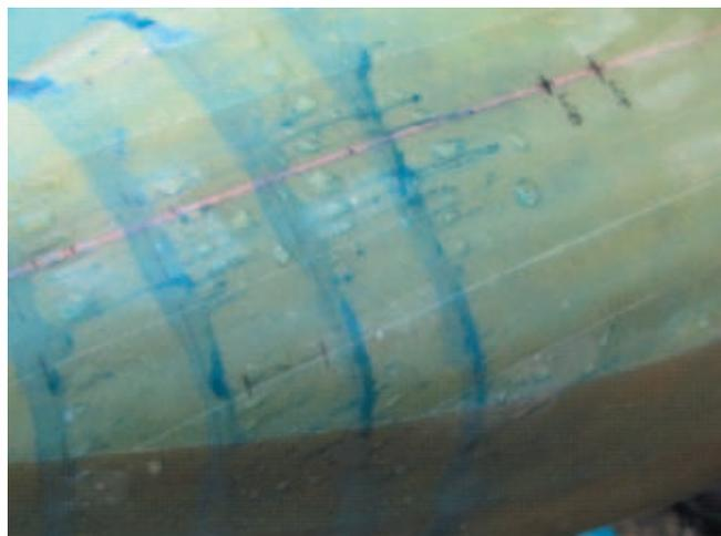
By using dye lines and then towing the model the flow streams could be established.
