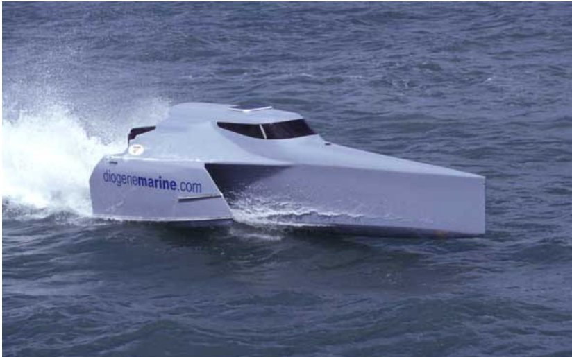
Fig 1 – 6m Wavepiercer Trimaran Proof of Concept Model (photo credit Geoff Green)
