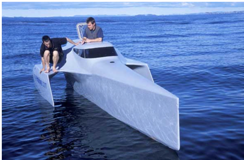
Fig II – One man on the gunwhale and negligible roll angle (photo credit Geoff Green)
