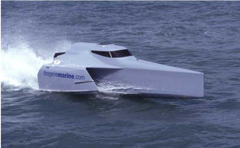
Fig 1 – 6m Wavepiercer Trimaran Proof of Concept Model (photo credit Geoff Green)
