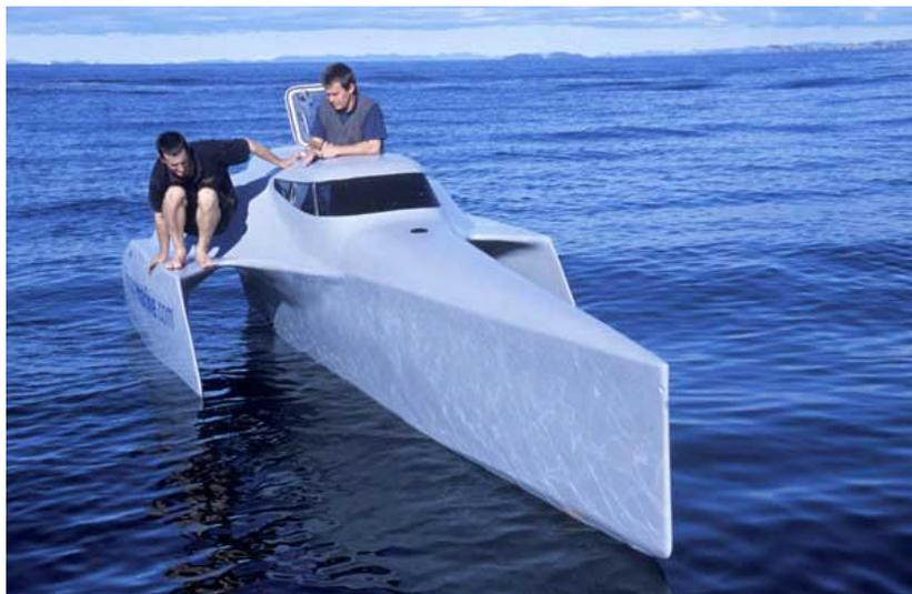
Fig II – One man on the gunwhale and negligible roll angle (photo credit Geoff Green)
