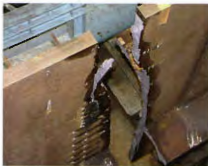
Typical brittle fracture propagated in thick base plate (ESSO test).
