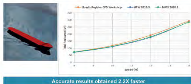
Figure 3: Results from MMS benchmark test using the Lloyd’s Register MV Regal
