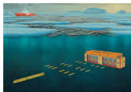
Figure 1 - General view of a group of AUVs launched from the robotic system to form a seismic signal recording platform
