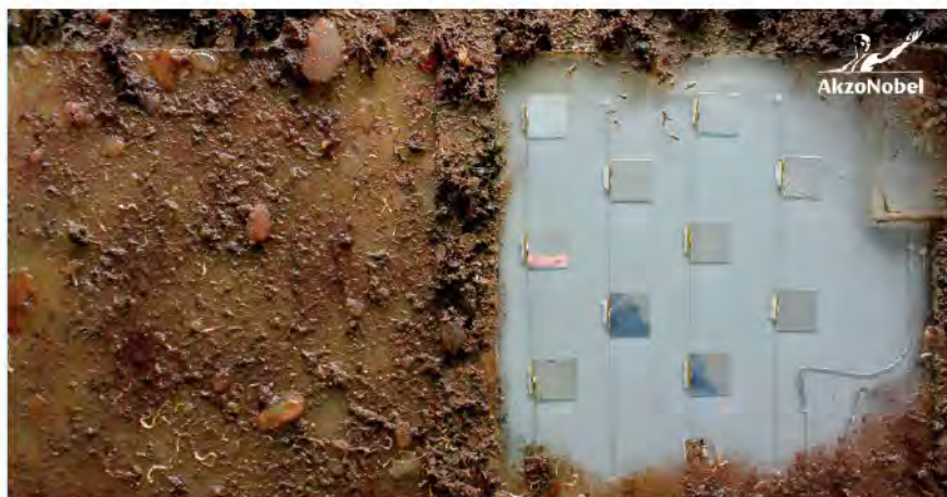
Embedded LEDs prevent fouling through UV light – clever (Philips)
