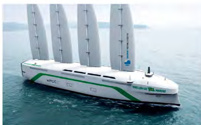
Becker Marine Systems bets on sails and hydrogen for zero-carbon shipping (Becker Marine Systems)
