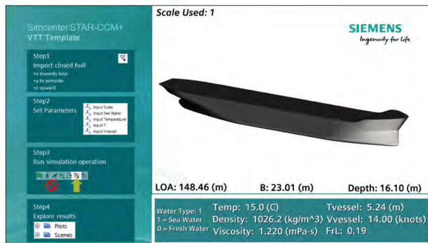
Figure 1: Setup via a template reduces set up time to minutes and ensures consistent set up of simulations
