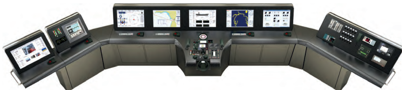
Synapsis Bridge Control is Raytheon Anschütz's latest generation Integrated Navigation System
