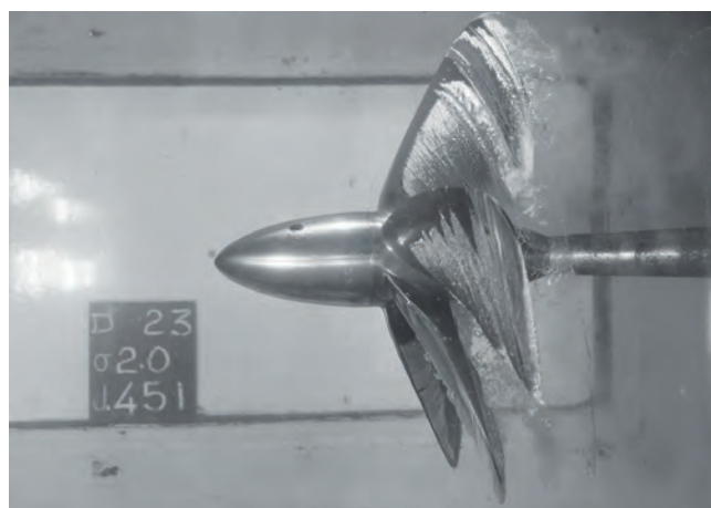
Figure 5. Meridian propeller series performance data (KT, 10KQ, \eta_o ), for varying Pitch / Diameter ratio and cavitation pattern in tunnel test
