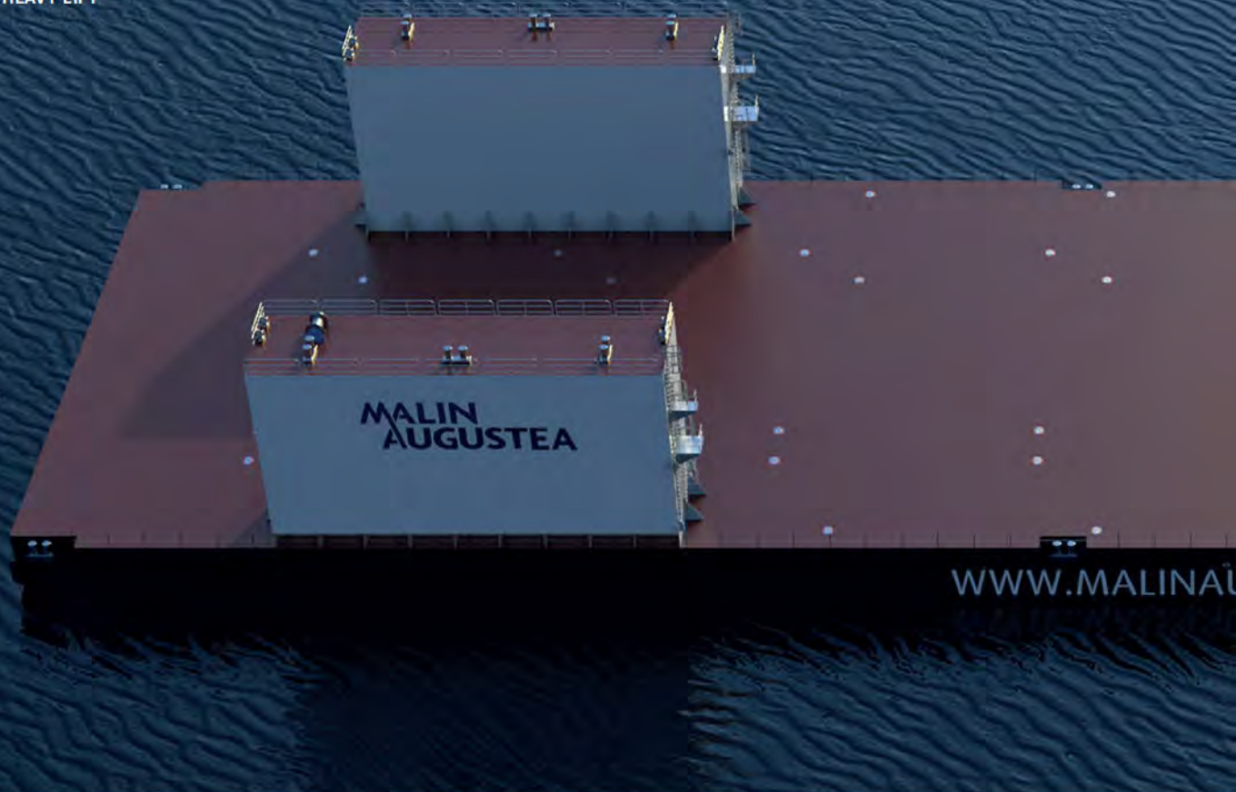
MALIN'S SEMI-SUB BARGE FOR THE T26 PROJECT. SOURCE: MALIN ABRAM
