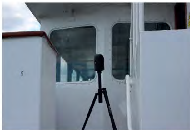
SCANNER ONBOARD THE HDS SCANNER CURRENTLY ONBOARD A VESSEL
