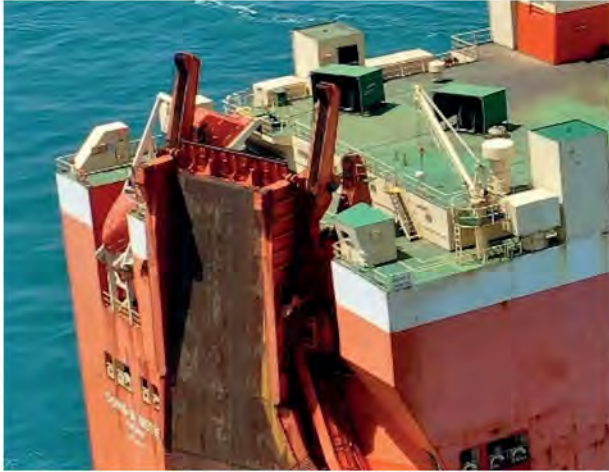
FIG. 1. IMAGINE THIS SHIP WITH LARGE HEEL TO STARBOARD AND TRY TO REACH THE FREE-FALL LIFEBOAT. THE INCLINING TEST COULD BE A GOOD OPPORTUNITY TO CHECK SUCH POSSIBILITY.
