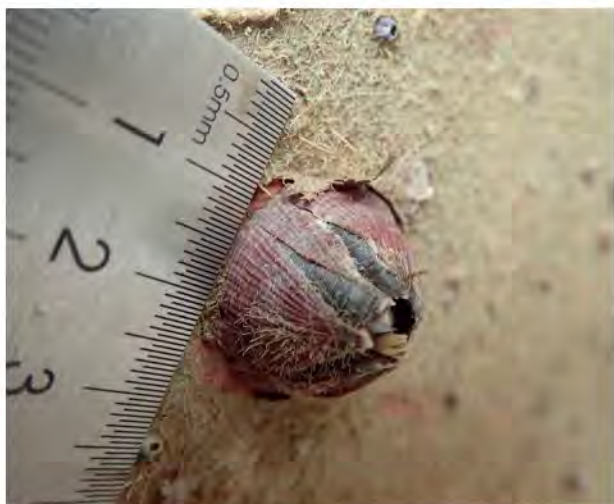
FIG. 1: EXAMPLE OF ANIMAL FOULING ON ARRIVAL AT DRYDOCK. SOURCE: SAFINAH GROUP
