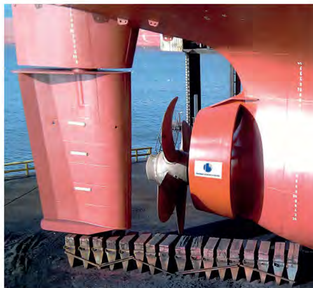
PROPELLER BULBS, SUCH AS THE MEWIS DUCT, CAN IMPROVE EFFICIENCY IN THE EVENT OF ADOPTING POWER LIMITING TECHNOLOGY
