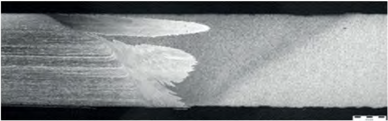
FIG. 6: METALLOGRAPHIC SECTION THROUGH A WELD MADE BETWEEN 8MM THICK S355 CARBON STEEL AND S32205 DUPLEX STAINLESS STEEL
