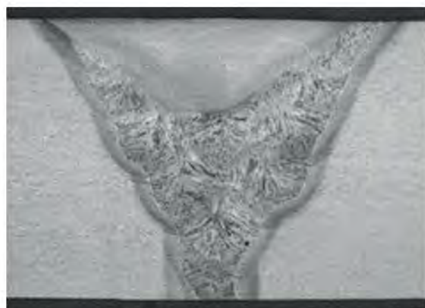
FIG. 2: A METALLOGRAPHIC SECTION THROUGH A MULTI-PASS ARC WELD IN 20MM THICK CARBON STEEL, WITH THE WELD CAP RE-PROCESSED BY FSW TO SHOW THE DIFFERENCE IN WELD MICROSTRUCTURE
