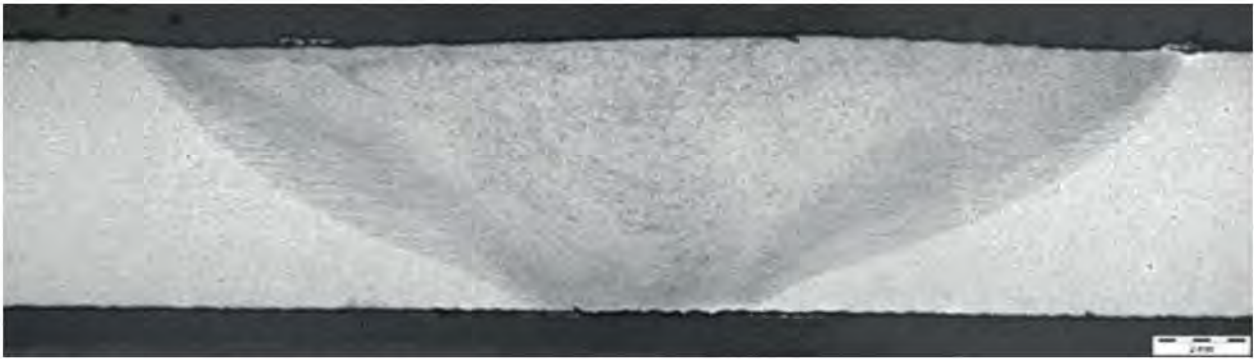
FIG. 3: A METALLOGRAPHIC SECTION THROUGH A SINGLE PASS FSW IN 6MM THICK DH36 STEEL
