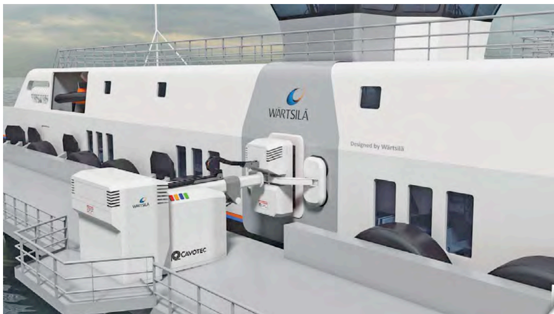
The Wärtsilä/Cavotec charging station powering Wärtsilä’s new ferry concept
