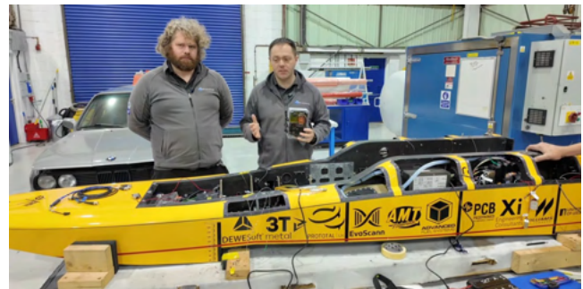
The quarter scale C3.2B composite model with a glimpse of the on-board control and monitoring systems. The jet engine had been removed (Screenshot courtesy of ThrustWSH team video)
