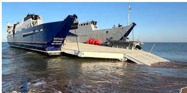
The stern landing vessel Matilda 1 with her stern ramp lowered during beach landing trials at Dundee Beach, Northern Territory, July 8, 2026 (Photo courtesy Seatransport)
