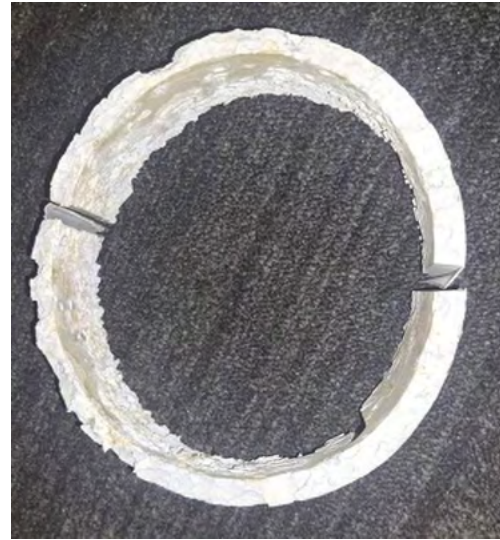
Figure 27 – Sacrificial sleeve mating face with bearing recess 22M Corrosion
