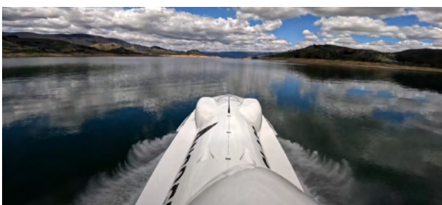
Spirit of Australia 2 tailplane video camera footage screenshots from August 2025 trials on Blowering Dam showing oscillation of spray sheets from the forward hydroplanes (Courtesy Warby Motorsport team Facebook page video)
