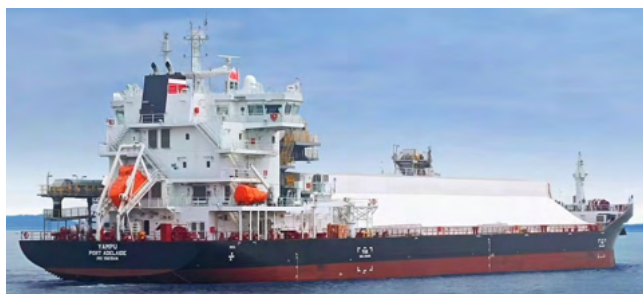
Yampu battery hybrid limestone carrier (Photo courtesy CSL Group)
