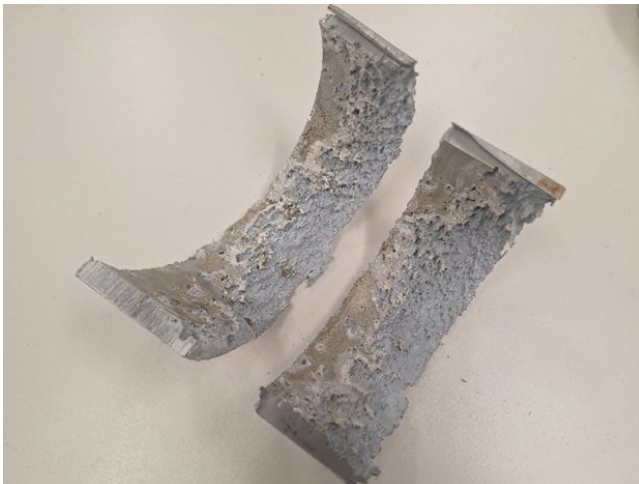
Figure 1 – Forward Sacrificial Sleeve Insert removed after 22 months of installation
