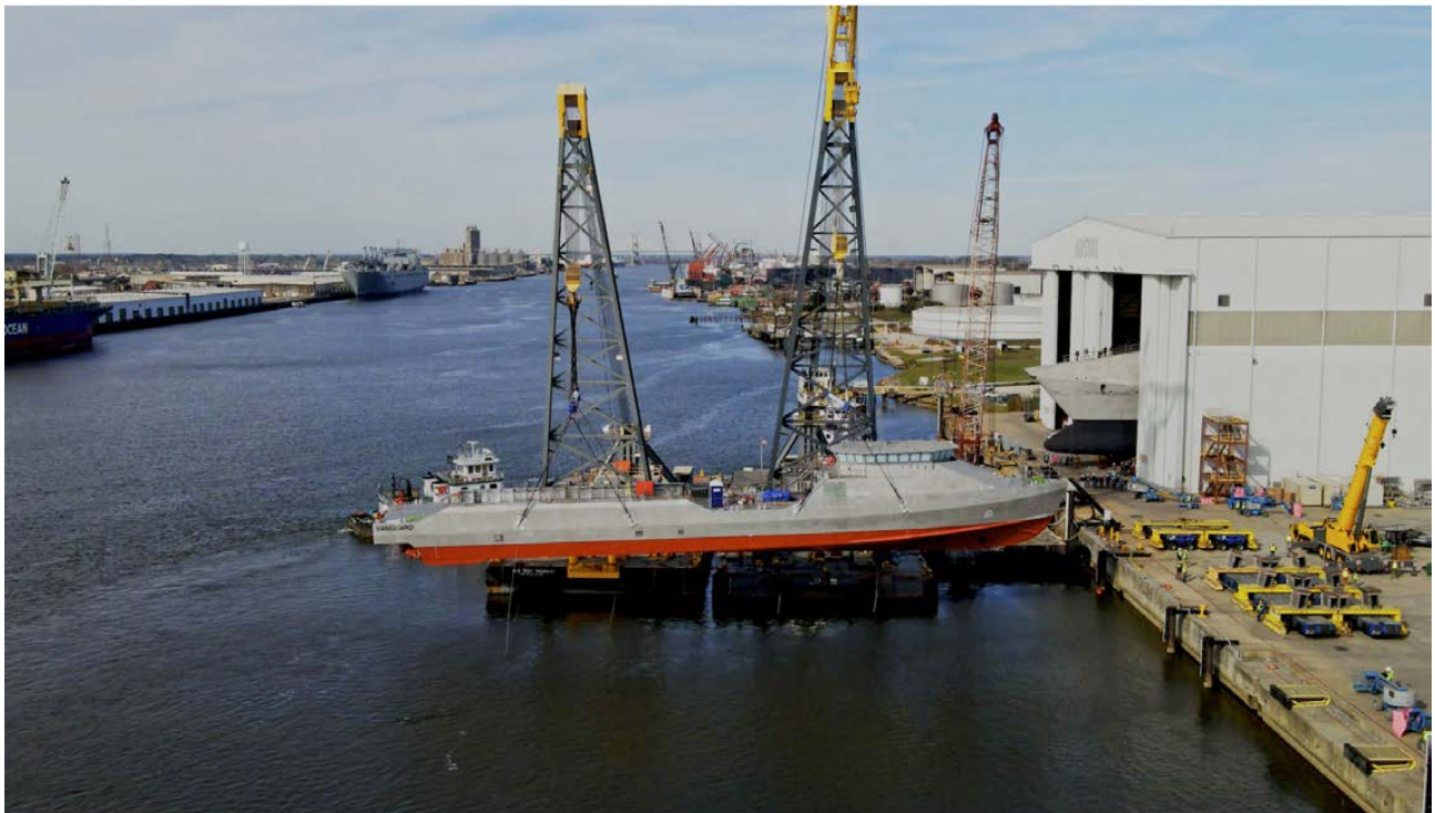
The launching at Austal USA of Vanguard (OUSV3), the first US Navy vessel purpose-built for autonomous operations from the keel up. Vanguard is being jointly developed by a team led by Austal USA and L3Harris (US Navy photograph)
