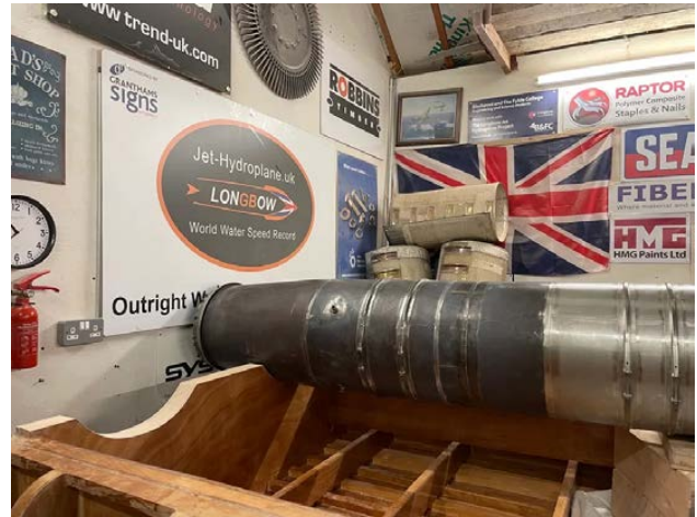
Jet exit pipes fitted to the transom on Longbow (Photo from Longbow website)
