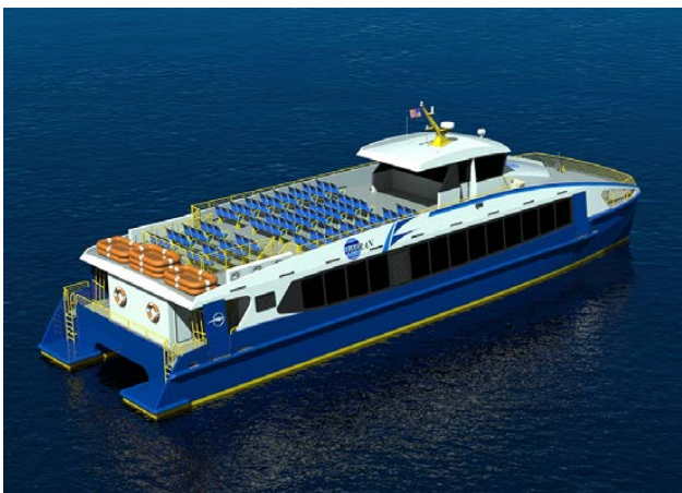
Starboard quarter of 32 m passage ferry for US Virgin Islands (Image courtesy Incat Crowther)
