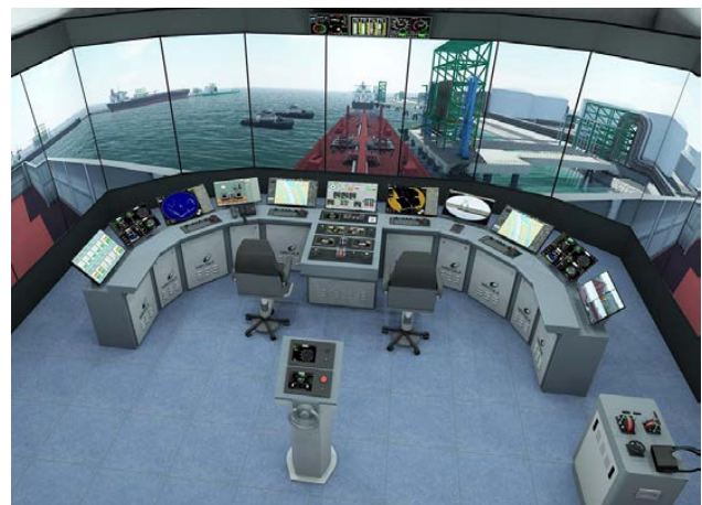
The new Wärtsilä simulator will feature the latest versions of Wärtsilä’s Navi-Trainer professional and Techsim simulation software, as well as the latest Navi Sailor and NACOS Platinum bridge systems. These include multi-pilot workstations for ECDIS, radar and conning applications (Image courtesy Wärtsilä)
