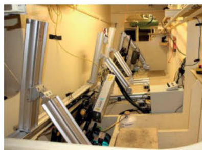
FIG. 5. PIV MEASUREMENT SETUP INSIDE THE STEERING GEAR ROOM, MV AMANDINE, KLEINWÄCHTER ET AL. (2015).
