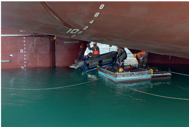
FIG. 13. REMOVING THE PIV UNIT WHILE THE VESSEL IS ALONGSIDE, 2022
