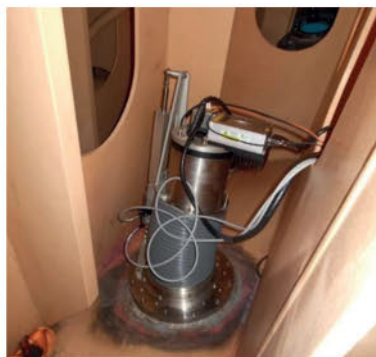
FIG. 4. LDV UNIT DURING FLOW MEASUREMENTS ON THE MV VALOVINE, PRINS (2015).
