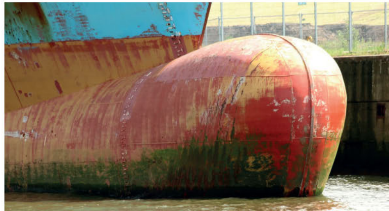
FOULING GROWTH ADDS SIGNIFICANT FRICTIONAL RESISTANCE TO VESSELS, RESULTING IN POOR ENERGY EFFICIENCY AND HIGHER CARBON EMISSIONS. SOURCE: GLOFOULING/IMO
