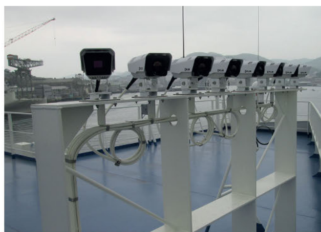
INFRARED CAMERAS ONBOARD SOLEIL DETECT OBSTACLES AND OTHER VESSELS. SOURCE: THE NIPPON FOUNDATION
