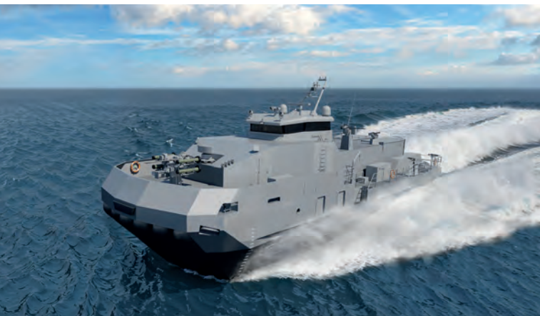
The Aircat Bengal MC uses a surface effect ship hullform, originally developed by ESNA in Norway
