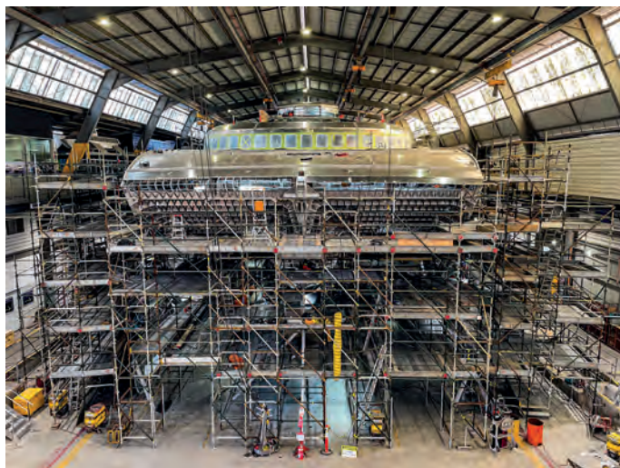
Work is now underway at Incat Tasmania's facility on Hull 100, a 78m-long hybrid fast ferry
