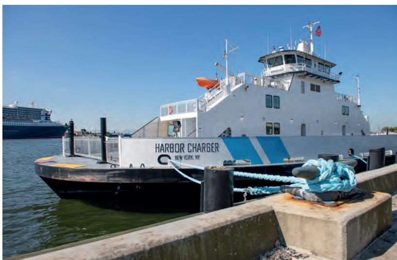
The 58m, steel ferry draws on a combination of CAT diesel gensets and Siemens BlueVault battery packs
