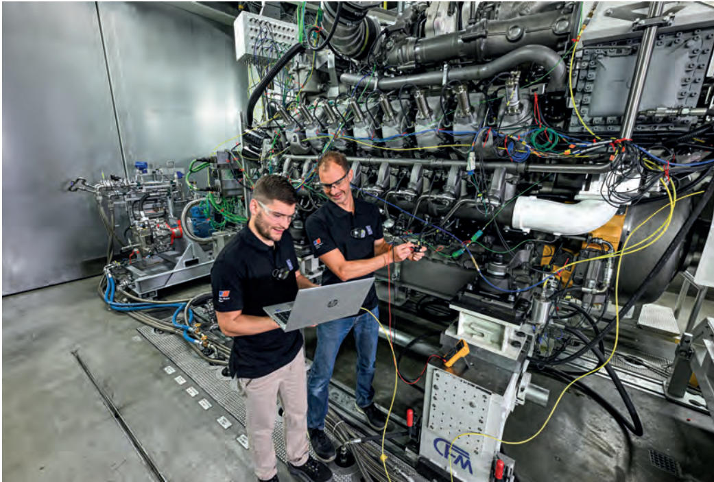
The first high-speed pure methanol engine has recently been tested on Rolls-Royce Power Systems' test bench in Friedrichshafen, Germany
