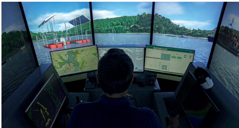
BMT's Rembrandt simulator was integrated with HydroSurv's vessel control software, enabling both remote operator training and direct control of the USV
