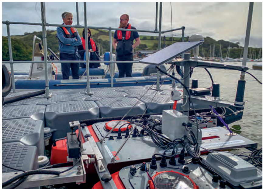
The prototype docking station, deployed on the River Dart in September, enables docking and recharging of South Devon College's USV Dart without manual intervention
