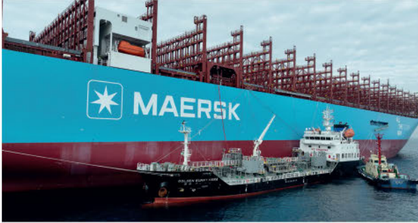
ANE MAERSK RECEIVING GREEN METHANOL FROM BUNKER TANKER GOLDEN SUNNY HANA. SOURCE: ULSAN PORT AUTHORITY
