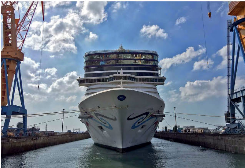
DAMEN'S DRYDOCK IN BREST CAN ACCEPT VESSELS DRAWING UP TO 13M OF WATER. SOURCE: ERWAN GUEGUENIAT/DAMEN SHIPREPAIR
