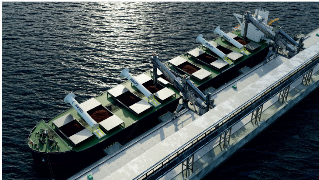
ANEMOI ROTOR SAILS FOLDING DEPLOYMENT SYSTEM. SOURCE: ANEMOI
