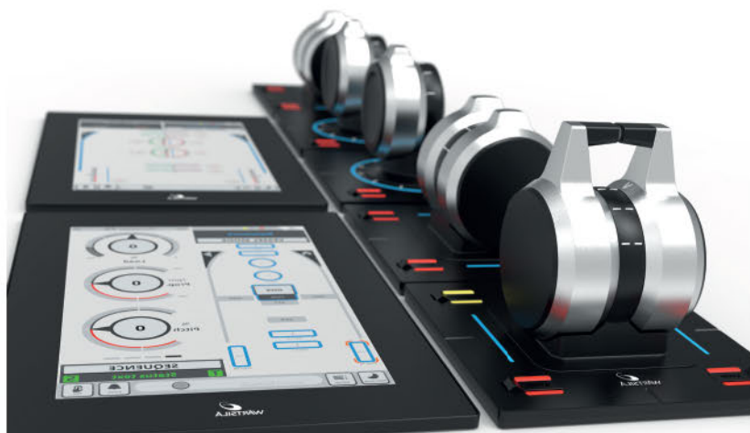
PROTOUCH REMOTE PROPULSION SYSTEM. THE SYSTEM REDUCES THE NEED FOR MULTIPLE SMALL DISPLAYS, STREAMLINING THE NUMBER OF TOUCH SCREENS USED AND MAKING EACH SCREEN LARGER
