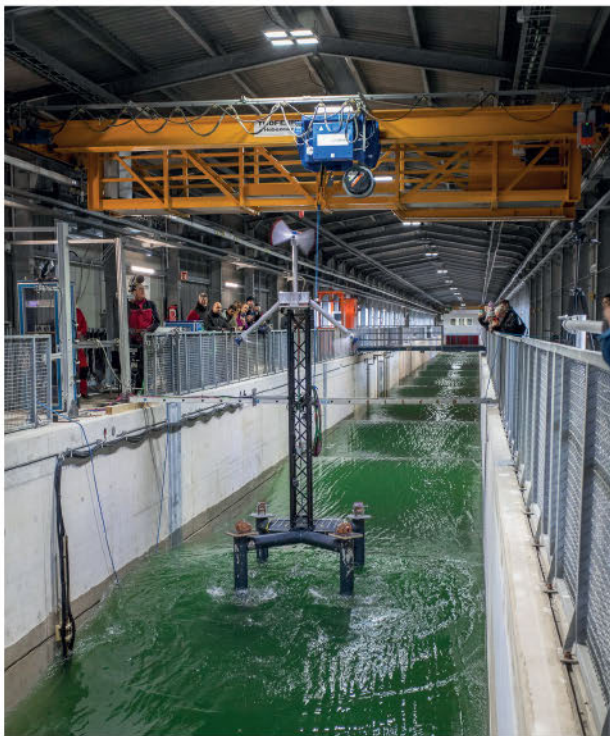
THE 1:15 SCALE FLOATING WIND TURBINE WAS CUSTOM MADE FROM ALUMINIUM AND IS BASED ON A REAL WIND TURBINE FROM PROJECT PARTNER GICON. SOURCE: MAX FUHRMANN/TU BRAUNSCHWEIG
