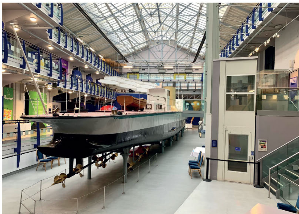
FIGURE 8. STERN VIEW OF SY TURBINIA IN THE DISCOVERY MUSEUM, NEWCASTLE-UPON-TYNE, IN 2024 SHOWING THE FINAL THREE-SHAFT AND NINE-PROPELLER CONFIGURATION AND PERSPEX HULL PANELS ALLOWING VIEWING OF THE THREE AXIAL-FLOW STEAM TURBINES AND OTHER MACHINERY
