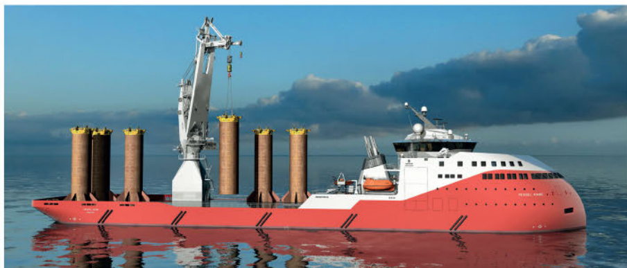
THE ULSTEIN SX232. DESIGNER'S ILLUSTRATION OF 6 X 20M SUCTION ANCHORS ON DECK. SOURCE: ULSTEIN
