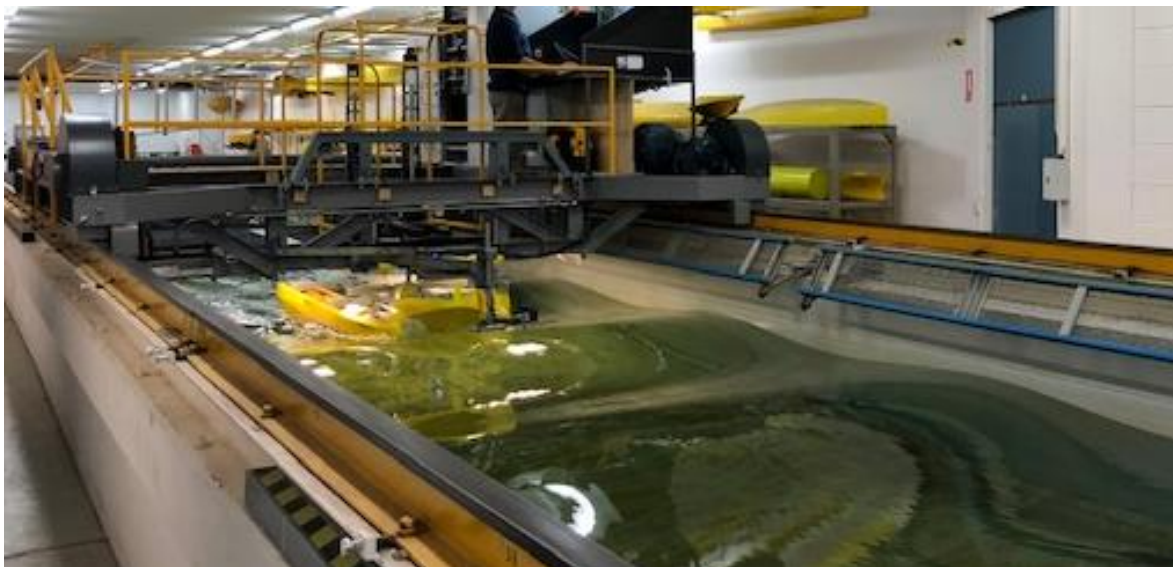
Figure 3: Showing the test model attached to the carriage of the towing tank facility at the Australian Maritime College, encountering a wave height of 72.7 mm at a speed of 1.53 m/s.
