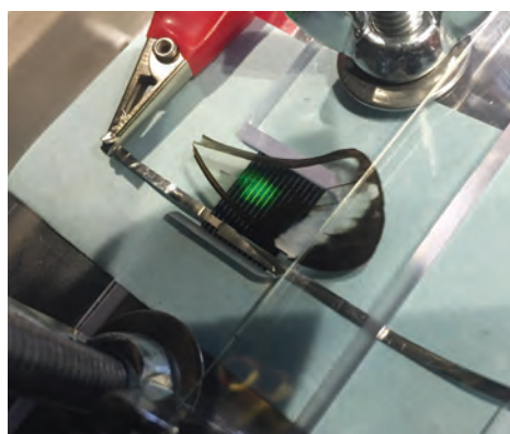
A 10mm x 10mm solar cell, developed in the first phase of the project
