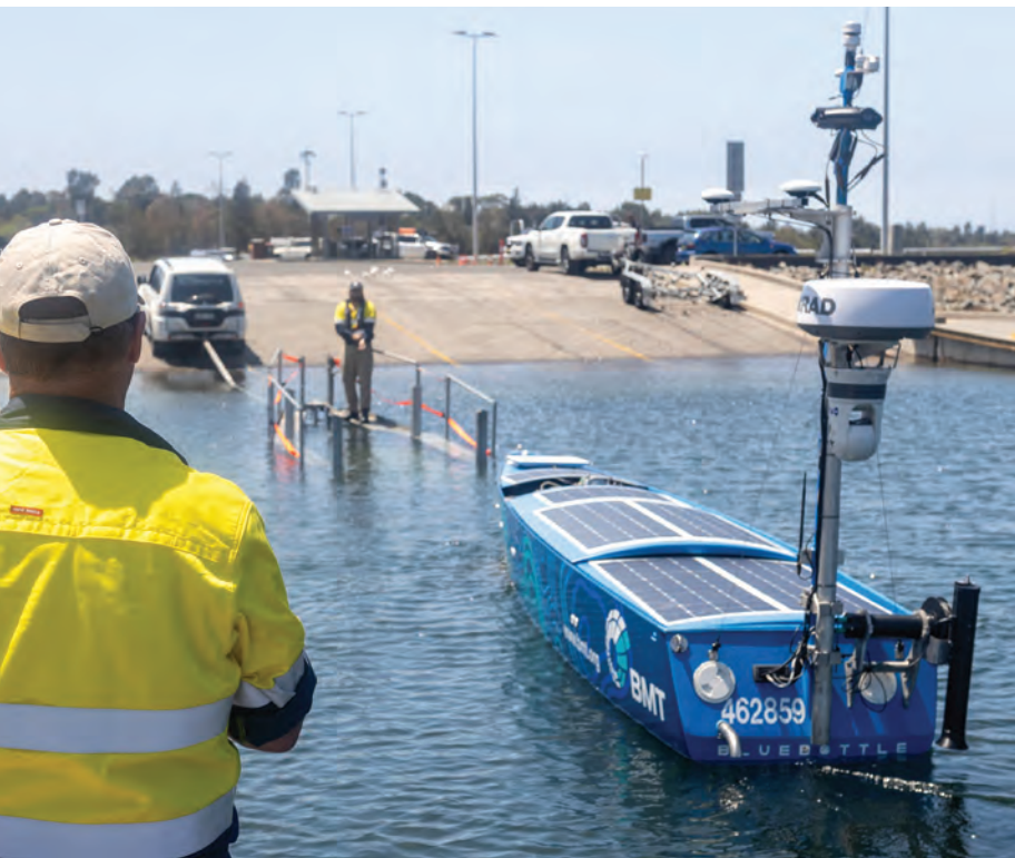
Left: The Deep Blue Project USV gathers real-time maritime data in coastal and offshore environments
