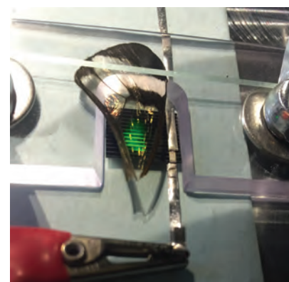
A 10mm x 10mm solar cell, developed in the first phase of the project
