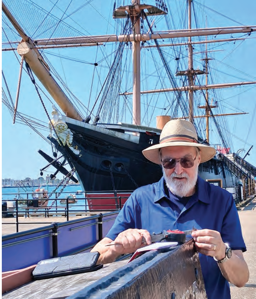
Robin checking the armour plate thickness of HMS Warrior (1860) at Portsmouth dockyard as part of a study of Victorian-era warships
