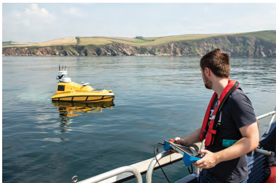
Left: Plymouth’s Cyber-SHIP Lab, used for assessing the cyber resilience of maritime vessels and their systems. Above: a student at Plymouth takes the controls of USV Cetus, a university vessel used for environmental monitoring and data gathering
