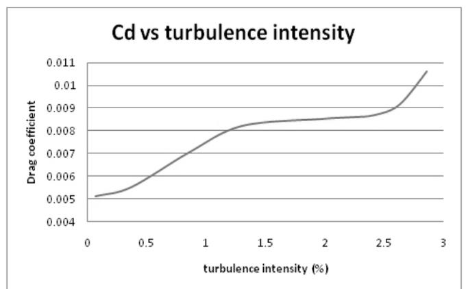
Figure 7: Graph showing the change in the drag coefficient of the keel section over a range of free-stream turbulence intensities, while operating in its representative upwind sailing condition
