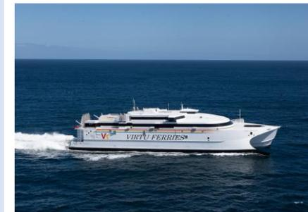
The new 110 metre RoPax ferry ordered by Virtu Ferrries, built by INCAT in Tasmania
