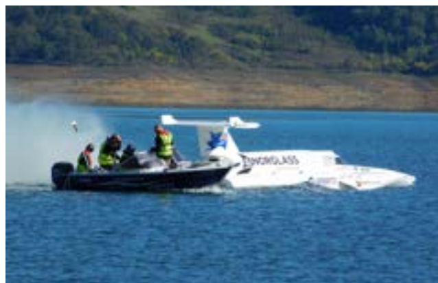
Spirit of Australia 2 shortly after engine startup with the assistance of crew and a battery bank on board one of the support boat at Blowering Dam on 31 August (Photo courtesy Martin Grimm)
