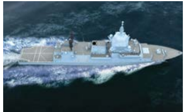
A bird's-eye view of the Hunter-class frigate, with the mast-mounted CEAFAR radar a major distinguishing feature.
