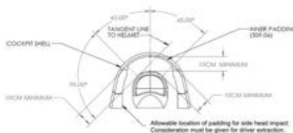
Illustration showing UIM cockpit clearance requirements around the drivers helmet (Image courtesy Longbow website)
