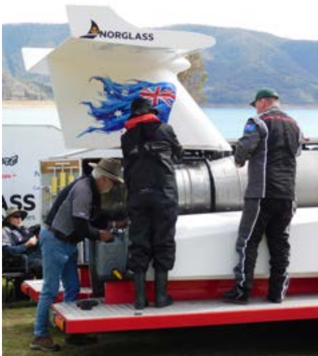
David and the team adjusting tailplane incidence angle of Spirit of Australia 2 at The Pines, Blowering Dam on 31 August (Photo courtesy Martin Grimm)
