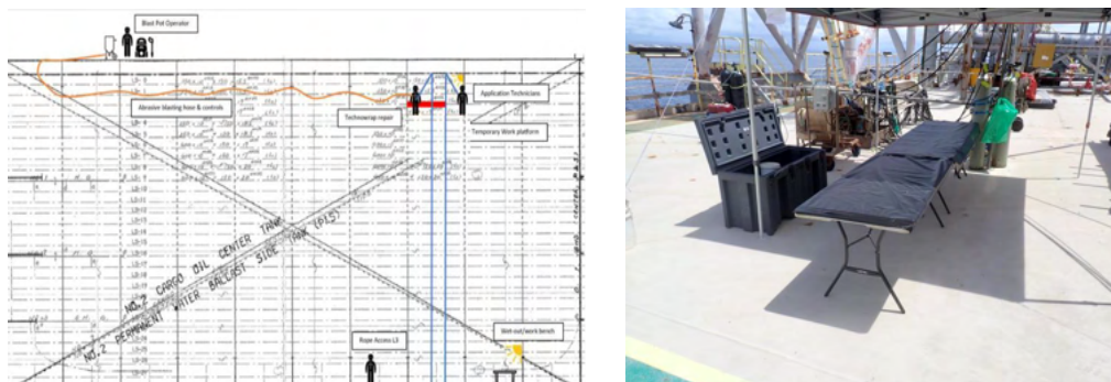
Figure 7 Locations of work front and wet out table set up on the main deck.
