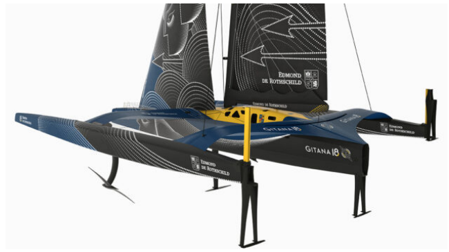
Gitana 18 illustration. Note 3 rudder foil sets (one retracted), main ama foils, canting centreline daggerboard T foil (Image courtesy Gitana team)
