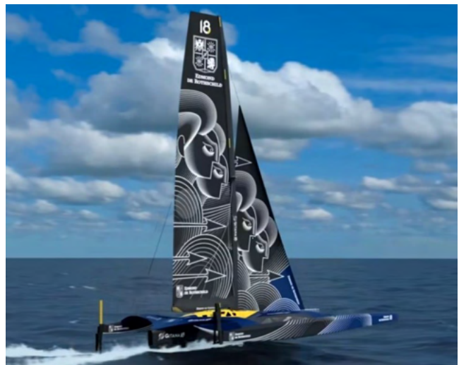
Image from animation of Gitana 18 underway foilborne showing the windward foils retracted to minimise drag (Image courtesy Gitana team video)
