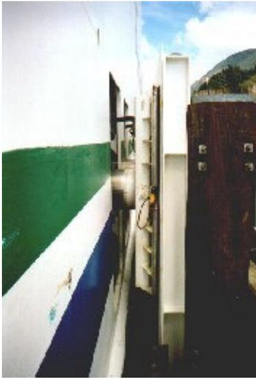
Fig 2 The Iron Sailor™ mounted forward on the port side of the Aratere in Wellington, NZ
