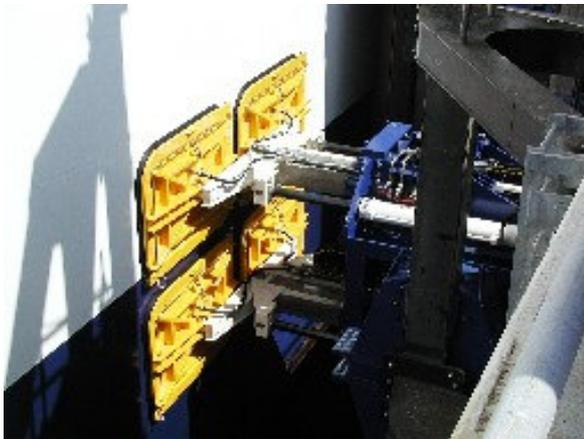
Fig 1- One of the 80 tonne Mooring System Ltd automated vacuum system which are installed for the Phase I development of the new Port of Dover
